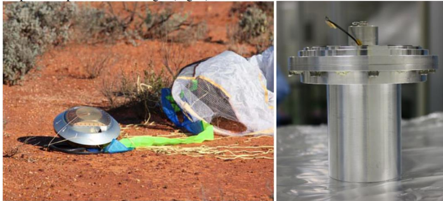
Figure 2-3 : Hayabusa sample return capsule after landing in Australia (Left) and Hayabusa sample container prior to opening (right) Image credit : JAXA
